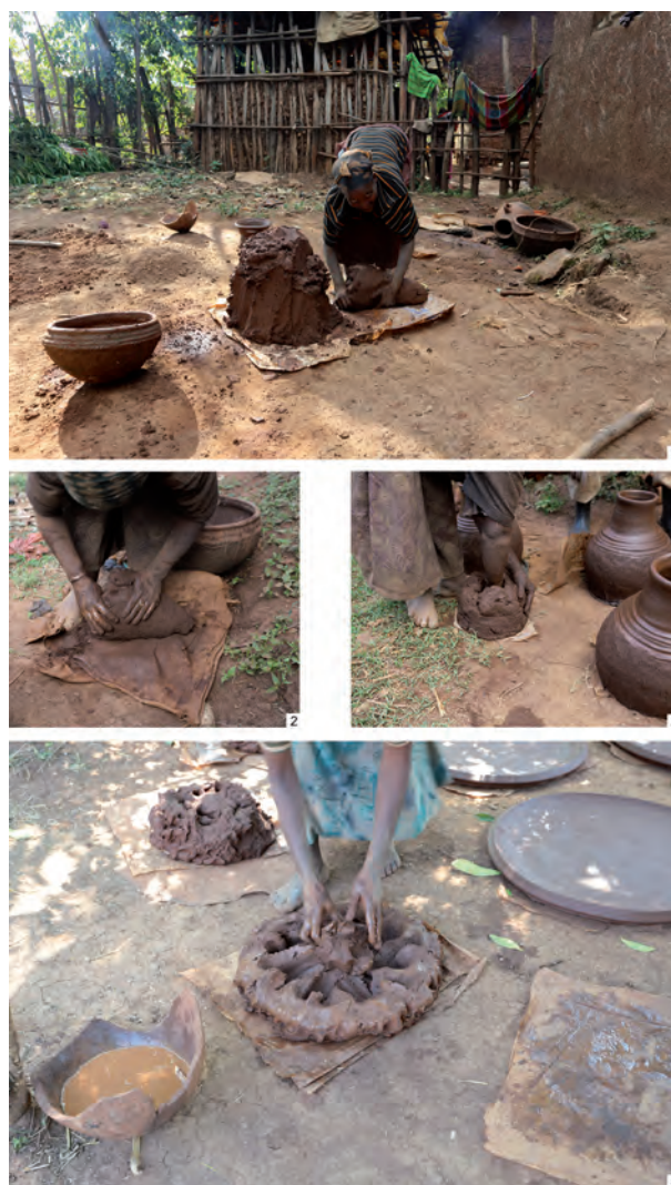
Fig. 18 – Woloyta social group at Goljoota. 1 and 2: shaping of a conical rough-out; 3: pinching of the rough-out; 4: shaping of an Ingera dish rough-out.
