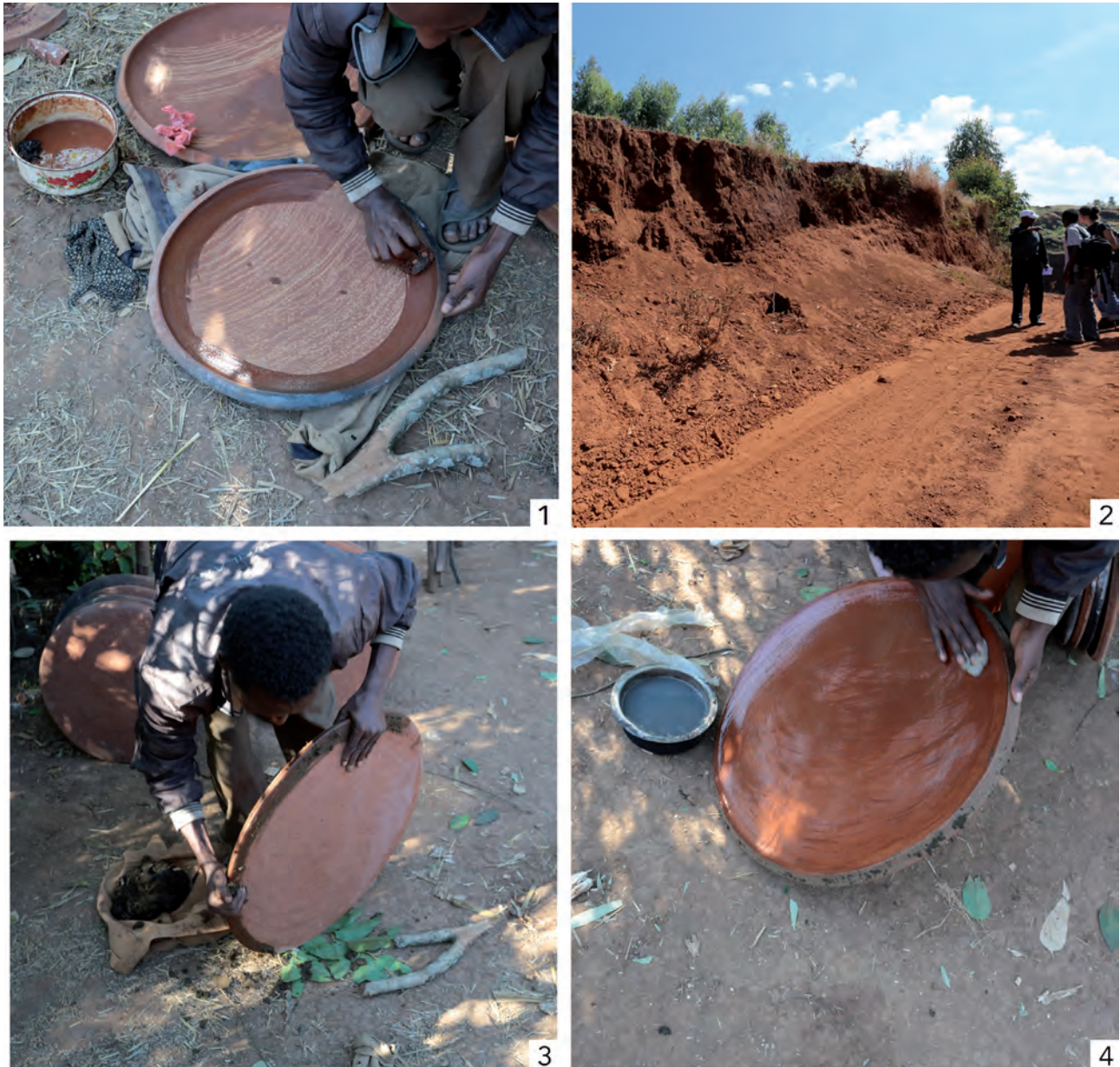
Fig. 17 – Woloyta social group at Goljoota. 1: spreading red slip or paint on the internal surface of an Ingera dish; 2: another extraction source of red clay used to make red paint which is applied after firing; 3: spreading animal dung on an Ingera dish edge; 4: spreading a mixture of Abyssinian banana tree roots and water on the internal surface of an Ingera in order create a shiny finish.
