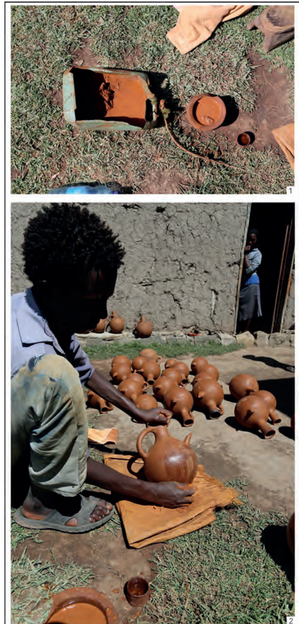
Fig. 16 – Oromo social group at Qarsa. 1: red clay is mixed with water and vegetable oil or diesel; 2: finishing stage used to create a shiny coating on Jabana (coffee pots).
