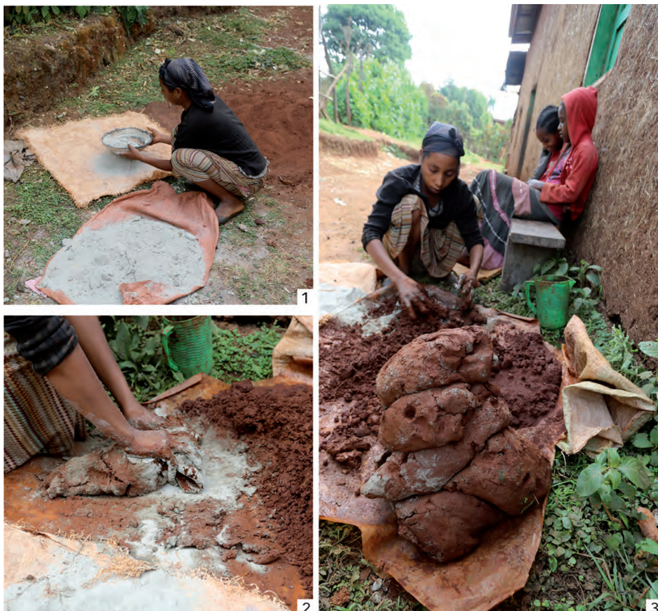
Fig. 12 – Oromo social group at Qarsa. 1 : sieving of white temper; 2: mixing of red clay and white temper; 3: shaping of small lumps of clay in preparation for roughing-out.
