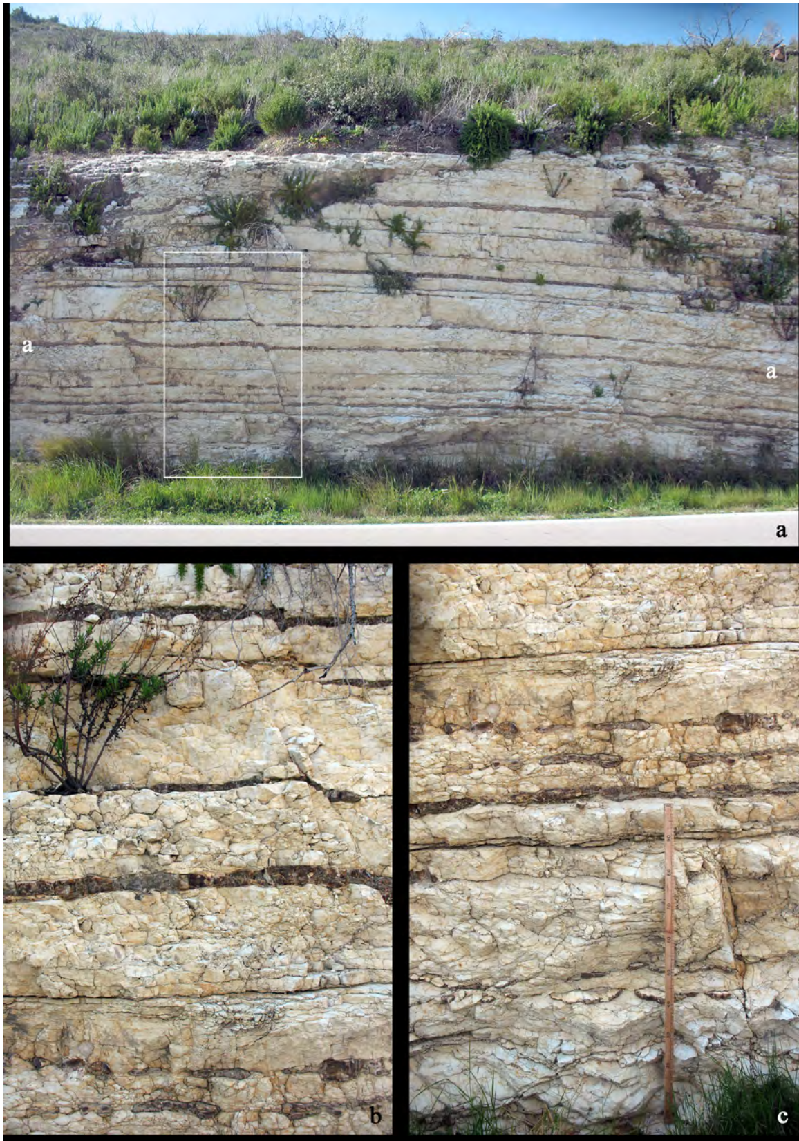
Fig. 5 – The road section at km 31 of the SP 53 'Mattinata-Vieste' road: nine specimens from the same horizontal layer (a), at a distance of 1 m, and eight specimens from eight layers arranged in a vertical sequence, were recovered from the area highlighted here by the white rectangle and illustrated by two details (b-c) of the upper and the lower part.
