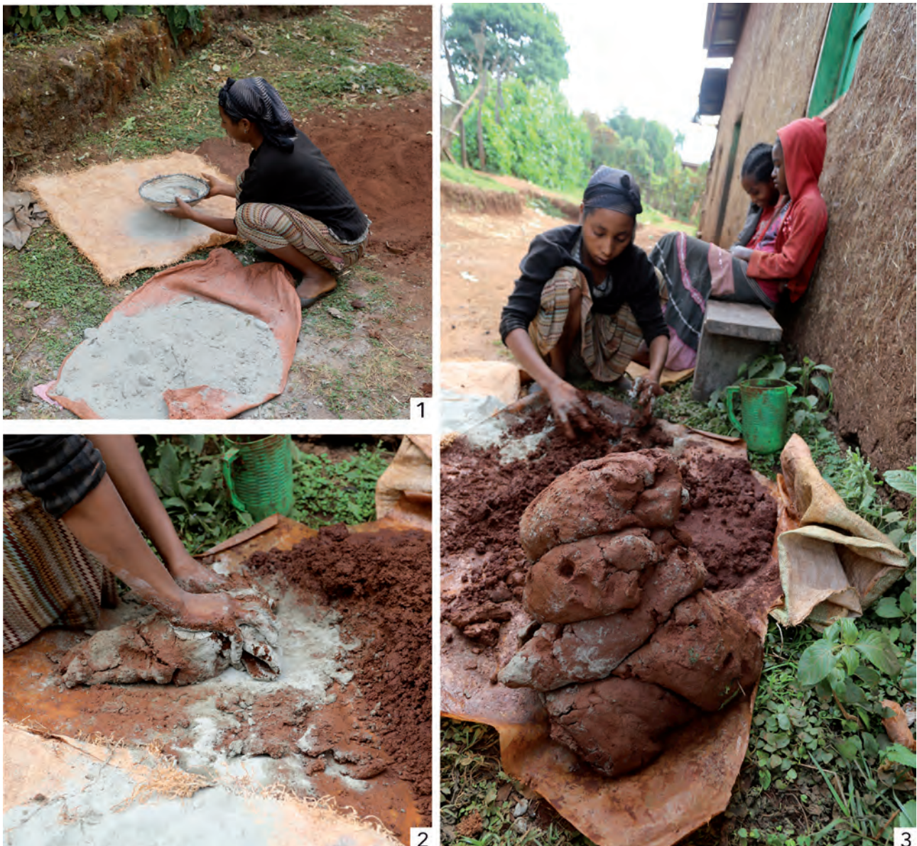
Fig. 12 – Oromo social group at Qarsa. 1 : sieving of white temper; 2: mixing of red clay and white temper; 3: shaping of small lumps of clay in preparation for roughing-out.
