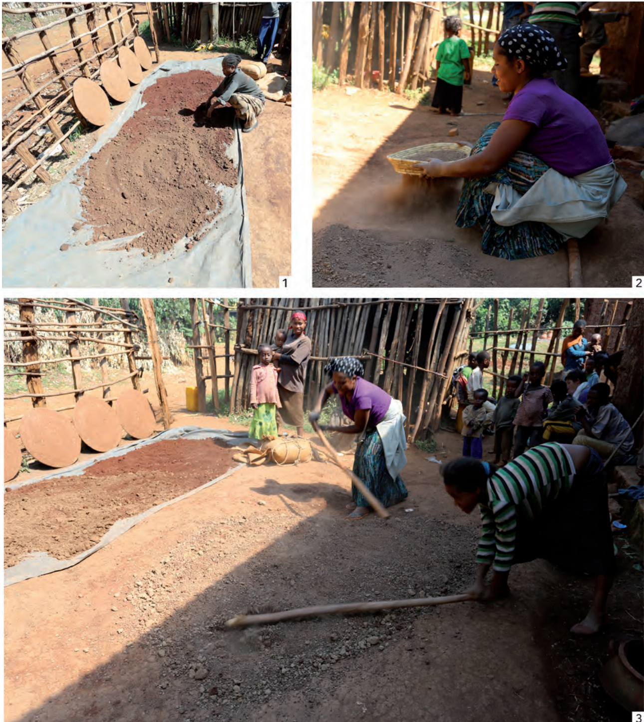
Fig. 9 – Woloyta social group at Goljoota. 1: drying of two clays; 2: sieving; 3: grinding with a pestle.
