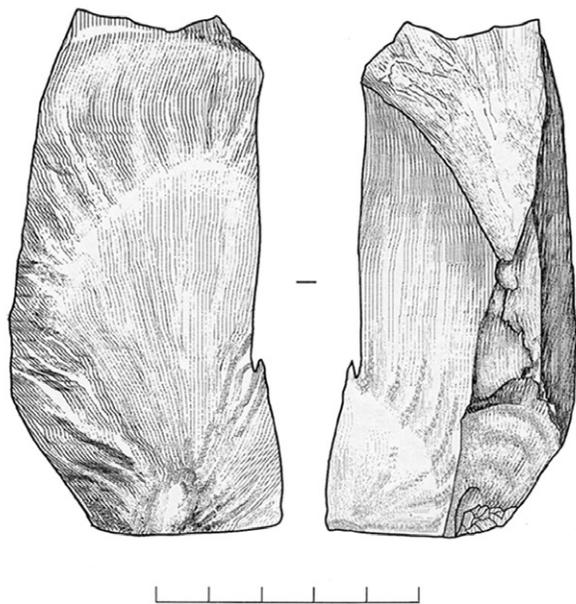
**Fig. 18** – Transverse flake removed from an ivory tusk frozen up to  $-40^{\circ}\text{C}$ , experiment carried out in 2007.
