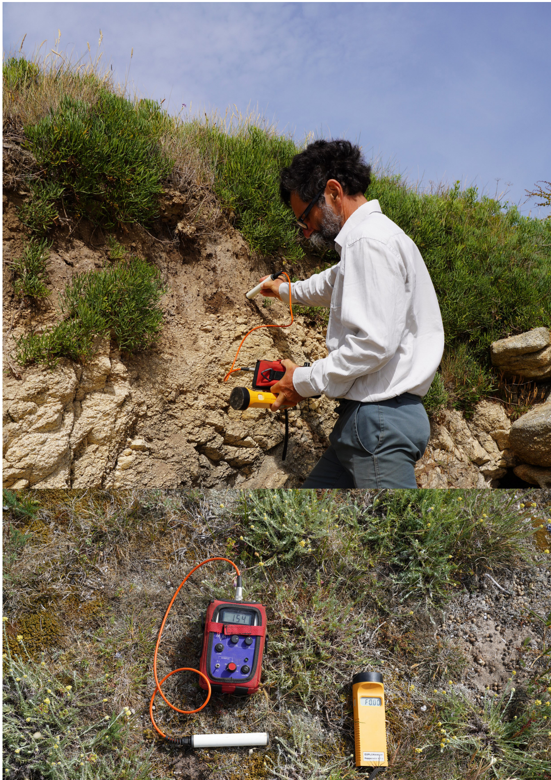
Fig. 10 – Recording of magnetic viscosity measurements with an MVM1 (Pulsepower Developments). The measurements are complementary to those made with the KT9 (Exploranium). Magnetic viscosity is an estimator of the concentration of nanometric magnetic phases (ferromagnetic in the broad sense, mainly ferrimagnetic), and is therefore independent of the low or non-magnetic matrix (paramagnetic or diamagnetic), unlike the measurement of magnetic susceptibility. The latter will be sensitive to the enhancement of the magnetic phase, mainly ferrimagnetic. These measurements were successively carried out on the same area (photo P. Arias).
