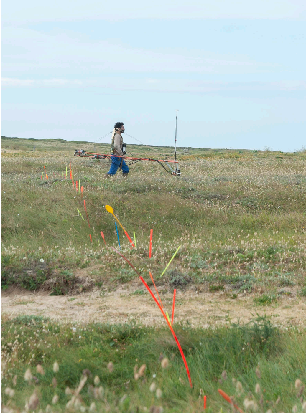
Fig. 1 – Device of realization of the geomagnetic prospecting on the Port Neuf site in Hoedic. The diagonal of coloured field markers planted in the ground corresponds to one of the parallel lines of visual markers placed every meter. The operator follows the alignment of the same coloured field markers, from one line of markers to the next, in order to cover the space evenly. The magnetometer's magnetic field intensity measurement sensors, shown here in the black of the GSMP-35G used, are placed at the front of the carrying structure. The GNSS antenna is offset above the sensors at the end of a pole so as not to pollute the magnetic field intensity measurements. The measurement acquisition console is carried against the operator's midriff. The electronic control units for the sensors and the battery are offset to the rear to limit the pollution from to their movement. This position also allows them to serve as a counterweight (photo P. Arias).
