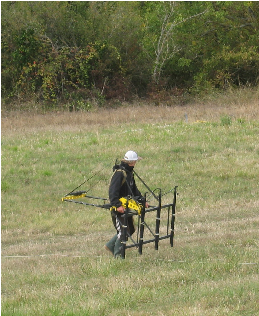
Fig. 3 – Vertical fluxgate gradiometer FEREX (Foerster Holding GmbH) with four sensors mounted on a carrying frame. The operator follows a line marked by a cord (photo V. Mathé).
